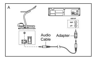
B. Plug one end of the audio cable into the jack on the side of the hiker near the power cord. Plug the other end of the cable into the included adapter. Plug the adapter into an RCA adapter (available at electronics stores). Next, remove the wire that is currently plugged into the AUDIO OUT jack on your VCR and plug the wire into the unused side of the RCA adapter. Plug the RCA adapter into the AUDIO OUT jack on your VCR.
